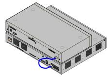
Any external expansion modules should be connected to the control unit before power is applied to the control unit. Ensure that modules are attached in the order that matches the planned or pre-built configuration.
