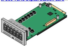
This card provides 8 TCM (digital station) ports for the connection of Avaya 4100, 7400, M-Series and T-Series phones.
