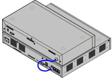
IP500 System with External Expansion Module
