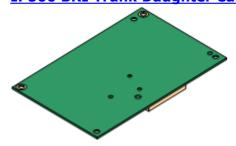
This card allows the base card to support up to 4 BRI trunk connections, each trunk providing 2B+D digital channels. The card is available in 2 port (4 channels) and 4 port (8 channels) variants.
