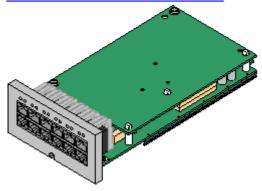
This card provides 6 digital station ports (1-6), 2 analog extension ports (7-8) and 2 BRI trunk ports (9-10, 4 channels). The card also includes 10 voice compression channels.
