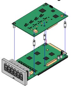
Most <u>IP500 base cards</u> 20 can be fitted with an IP500 trunk daughter cards to support the connection of trunks to the base card.
