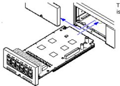
The IP500 base cards and trunk daughter cards should be fitted before power is applied to the control unit.
