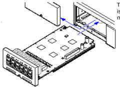
The IP500 base cards and trunk daughter cards should be fitted before power is applied to the control unit. Ensure that cards are inserted in the order that matches the planned or pre-built configuration.
