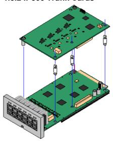
Most <u>IP500 base cards</u> 20 can be fitted with an IP500 trunk daughter cards to support the connection of trunks to the base card.
