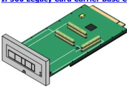
This card allows various IP400 trunk cards 24 and IP400 VCM cards 25 to be used. The front of the card includes panels that can be removed to match the trunk card fitted.
